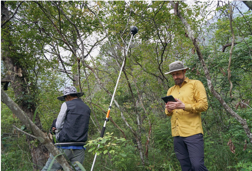
Fig. 32 Measuring the site Kharigup using differential GPS (photo C. Franken)
